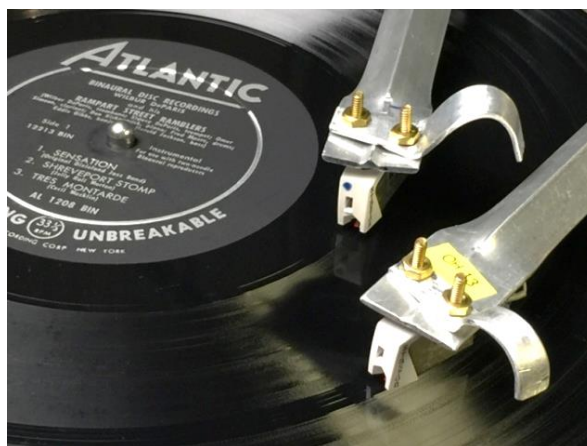
At the end of simultaneous replay of separate grooves by two transcription-length (305mm tip-to-pivot) tonearms to minimize dynamic speed variations. The ~136ms offset was lined up digitally. The pickups are Stanton 681\D6800SL Stereohedron.
